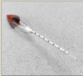
ASTM Soil Hydrometers ASTM D.422, E-100, AASHTO T-88.
